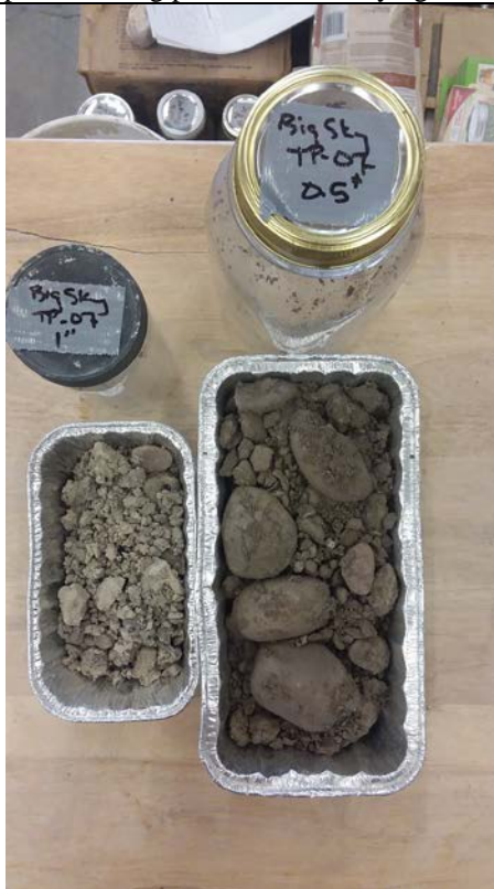
Description: TP-07 Moisture contents after being taken out of the drying oven.
