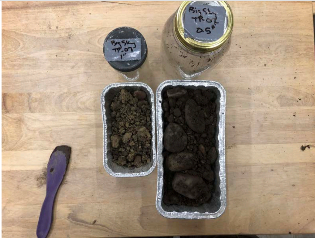
Description: TP-07 Moisture contents prior to being placed into the drying oven.
